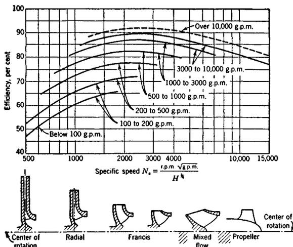
**Fig. 55.7** Variation of physical appearance and expected efficiency with specific speed for a variety of pump designs and sizes. (Courtesy of Worthington Corporation.)
