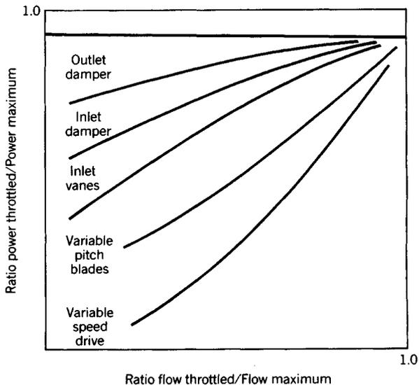
**Fig. 55.11** Effectiveness of various methods of controlling fans in variable volume service.
