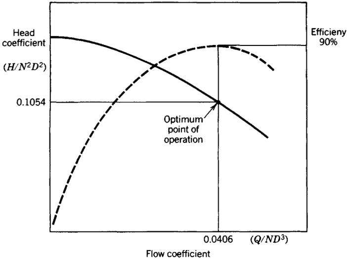
Fig. 55.8 Performance characteristics of a model pump, expressed nondimensionally.
