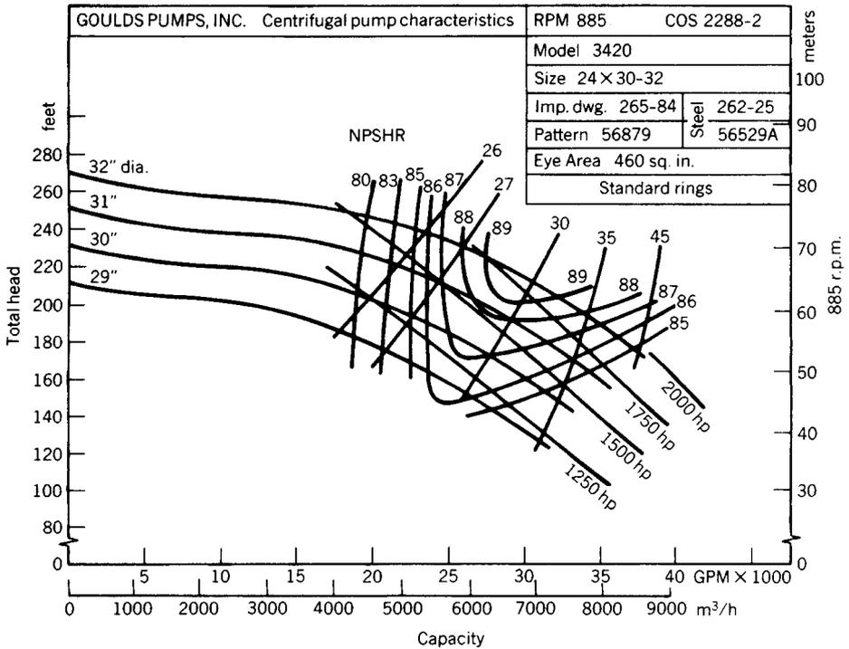
**Fig. 55.9** Example of pump curve provided by manufacturer. (Courtesy Goulds Pumps, Inc., Seneca Falls, NY.)
