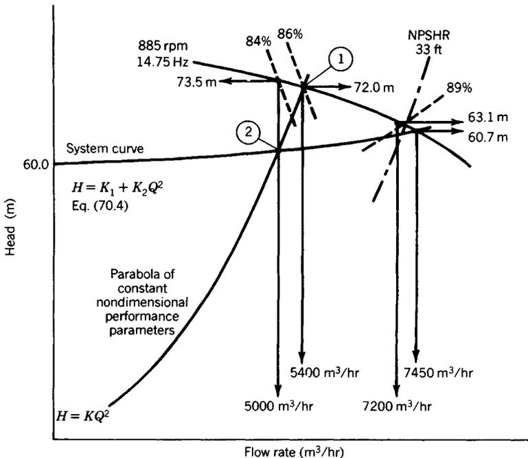
Fig. 55.10 Point of operation of a pump in a system.
