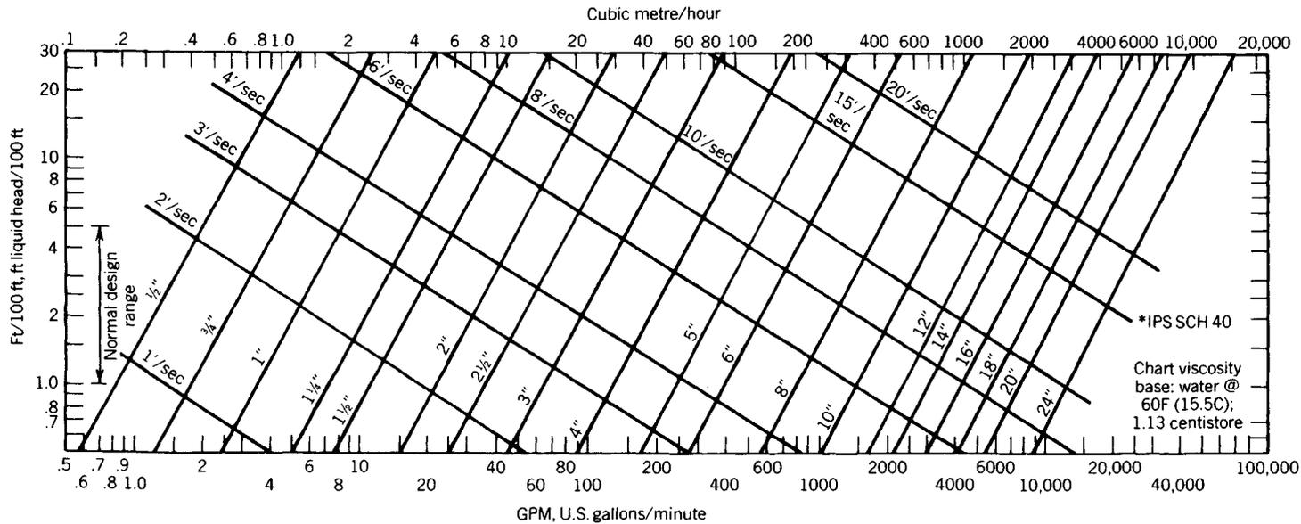
**Fig. 55.1** Friction loss for water in commercial steel pipe (schedule 40). (Courtesy of American Society of Heating, Refrigerating and Air Conditioning Engineers.)
