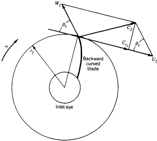
**Fig. 55.3** Relationships of velocity vectors used in Euler's theory for the developed head in a centrifugal fluid machine;  $W$  is the fluid's velocity with respect to the blade;  $\beta$  is the blade angle,  $\omega$  is the angular velocity, 1/sec.
