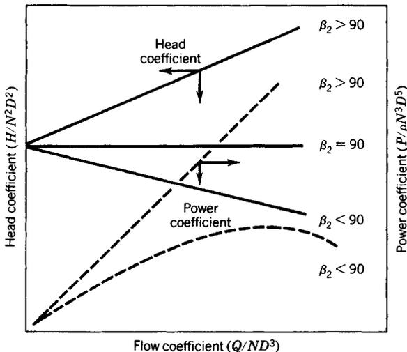
**Fig. 55.4** Theoretical (Euler's) head and power coefficients plotted against the flow coefficient for constant  $D/b$  ratio and for values of  $\beta < 90^\circ$ , equal to  $90^\circ$ , and  $> 90^\circ$ .
