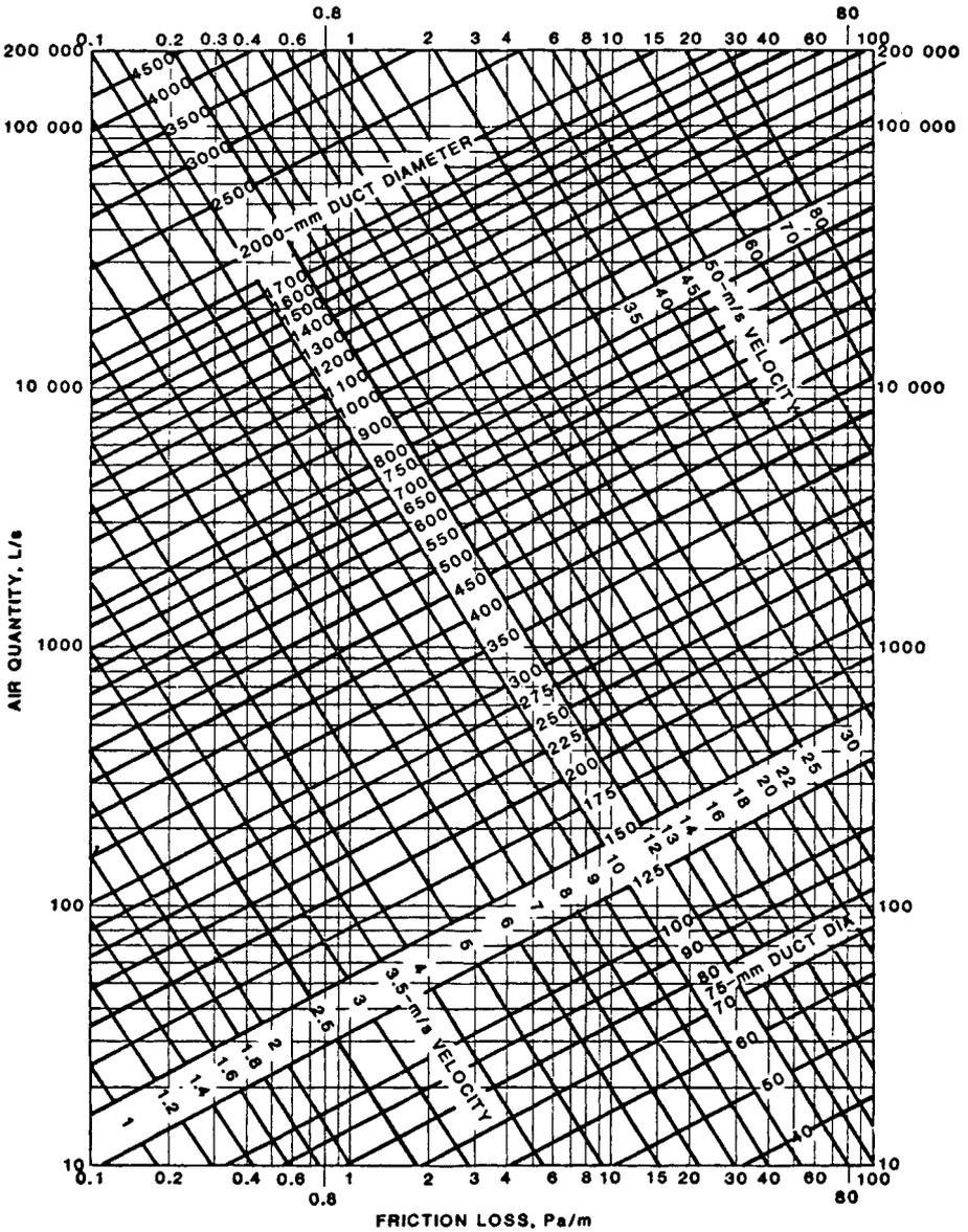
Fig. 55.2 Friction loss of air in straight ducts. (Courtesy of American Society of Heating, Refrigerating and Air Conditioning Engineers.)
