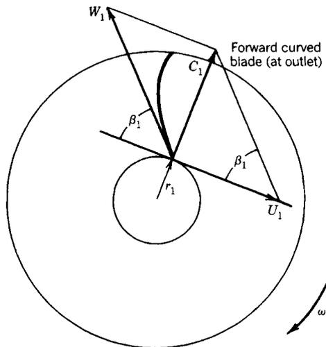
**Fig. 55.5** Relationship of velocity vectors at the inlet to the rotor. Symbols are defined in Section 55.3.1.
