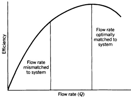
**Fig. 55.6** Typical efficiency curve for fluid machines of fixed geometry and constant angular frequency.
